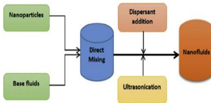
Fig 2.1.a:Preparation using Two Step Method
