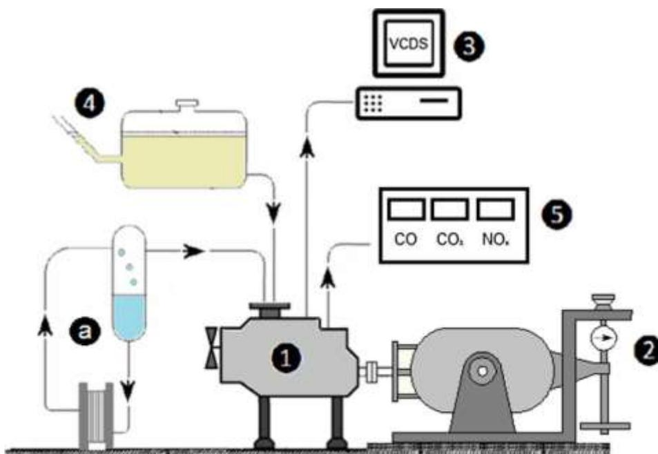
Fig-3: Schematic diagram of engine and test bed description.
