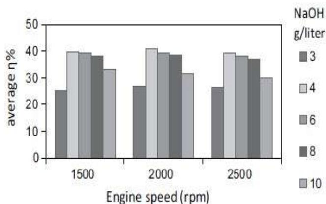
**Fig-5: Average efficiencies for using different concentrations of NaOH at different engine speeds.**
