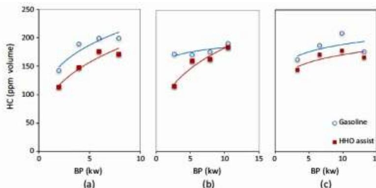
Fig. 10 Effect of varying the engine dynamometer load on HC emission
