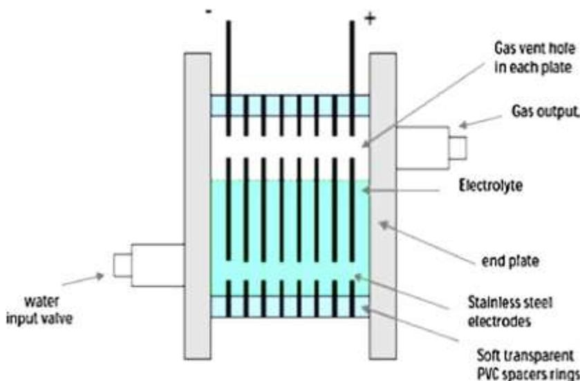
Fig-2: A schematic diagram of HHO dry cell
