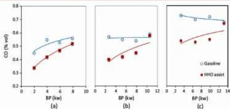
Fig-9: Effect of varying the engine dynamometer load on CO emission
