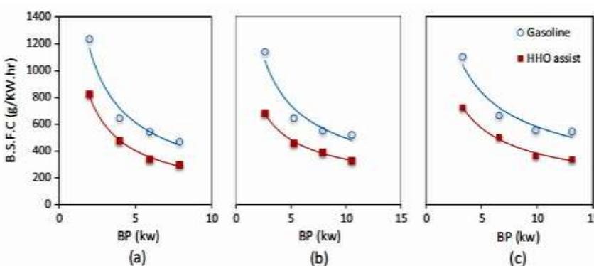
Fig-8: Effect of varying the engine dynamometer load on BSFC (a)1500rpm, (b)2000rpm and (c)2500rpm.
