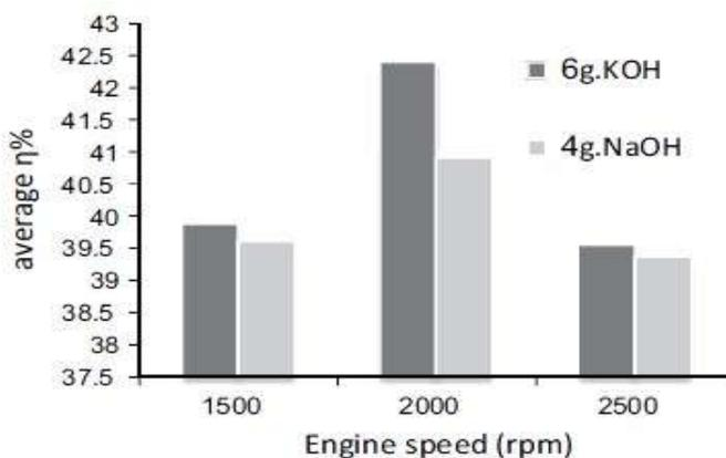
**Fig-6: Average efficiencies for using concentrations of 6g KOH and 4g NaOH per litre at different engine speed.**
