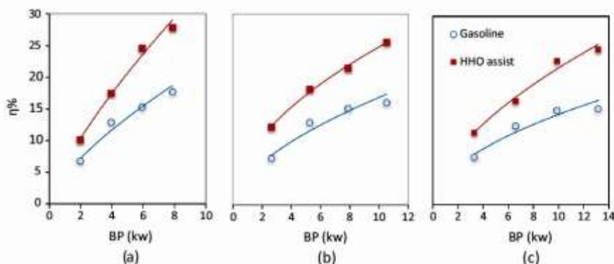
Fig-7: Overall thermal efficiency improvement with HHO over pure gasoline fuel at different engine speeds (a)1500rpm, (b)2000rpm and (c)2500rpm.
