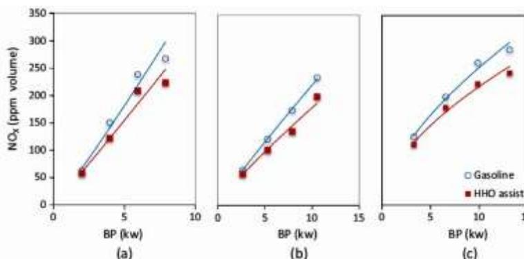
Fig-11: Effect of varying the engine dynamometer load on NOx emission
