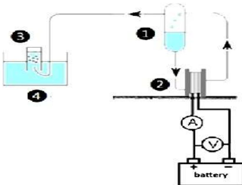
Fig-1: Schematic diagram of HHO gas generation system.
