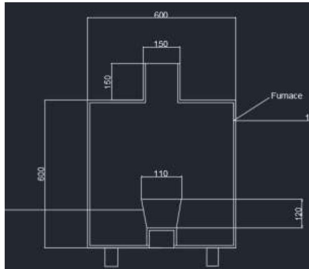
Fig 3. Furnace dimensions
