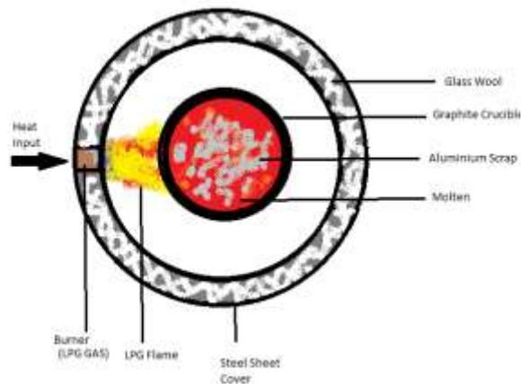
Fig 2. Melting operation
