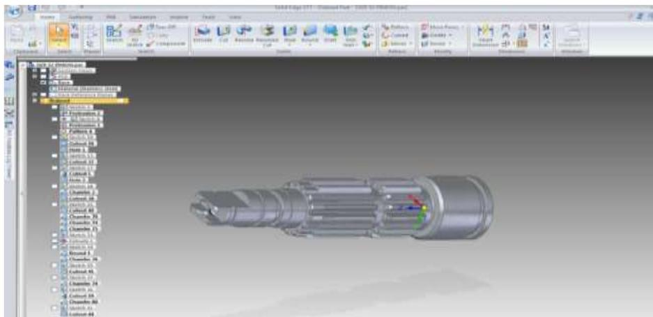
Fig.1 Actual Model in Solid Edge ST7
