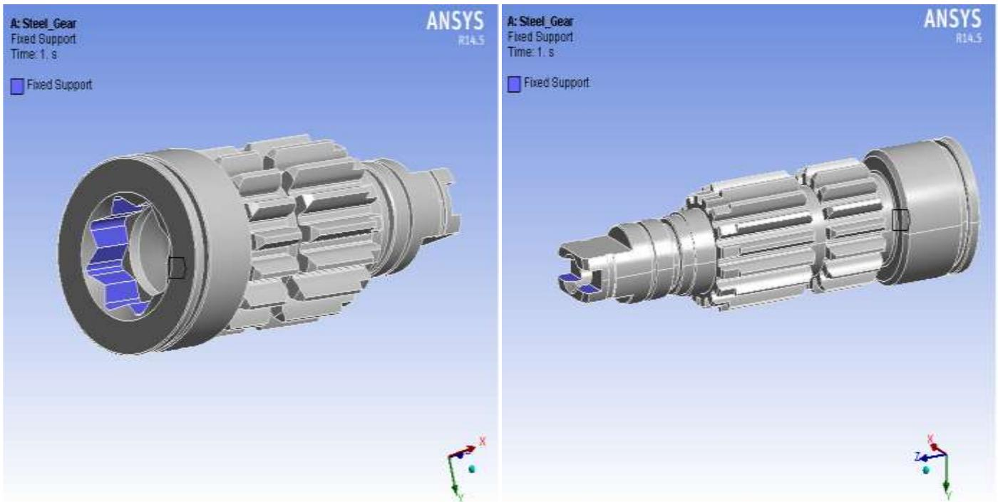
Fig 3- Loading And Boundary Conditions
