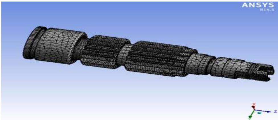
Fig.2 - Meshing of Spur Pinion
