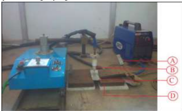
(A) Ground Clamp, (B) Work Stage, (C) Torch head assembly, (D) Work Piece
