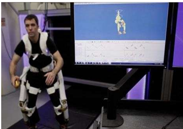
Exoskeleton to help paraplegics walk, derived from space robotic systems
