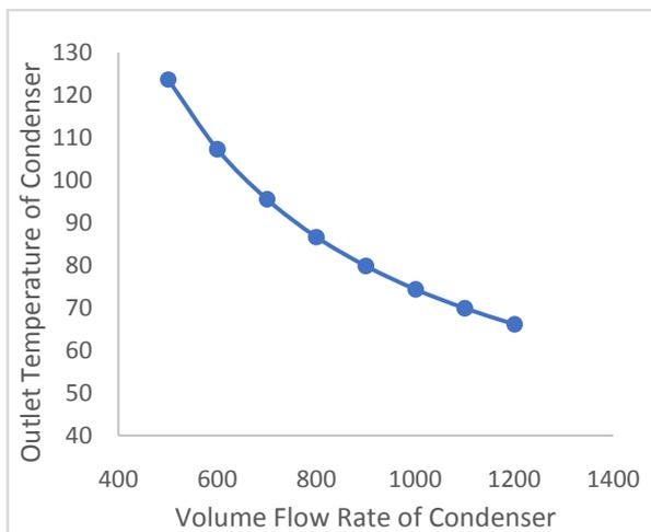
**FIGURE 6 THE EFFECT OF VARIOUS CONDENSER FLOW RATE ON THE OUTLET TEMPERATURE OF CONDENSER WHEN THE VOLUME FLOW RATE OF EVAPORATOR WAS KEPT CONSTANT AT 500 LPM**
