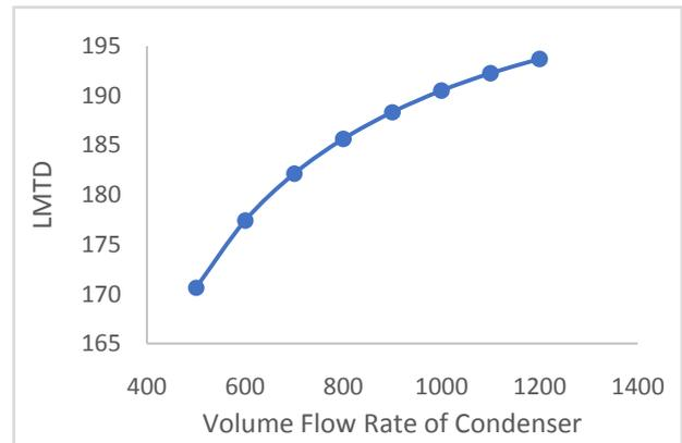
**FIGURE 7 THE EFFECT OF VARIOUS CONDENSER FLOW RATE ON THE LOG MEAN TEMPERATURE OF HEAT EXCHANGER WHEN THE VOLUME FLOW RATE OF EVAPORATOR WAS KEPT CONSTANT AT 500 LPM**
