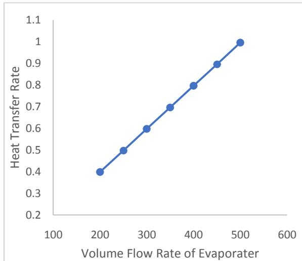
**FIGURE 5 THE EFFECT OF VOLUME FLOW RATE OF EVAPORATOR ON THE HEAT TRANSFER RATE WHEN THE CONDENSER VOLUME FLOW RATE IS ALSO VARIED**
