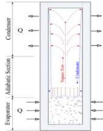
FIGURE 1 SCHEMATIC REPRESENTATION OF HEAT PIPE
