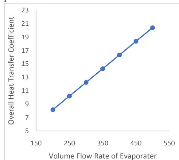
FIGURE 4 THE EFFECT OF VOLUME FLOW RATE OF EVAPORATOR ON THE OVERALL HEAT TRANSFER RATE WHEN THE CONDENSER VOLUME FLOW RATE IS ALSO VARIED
