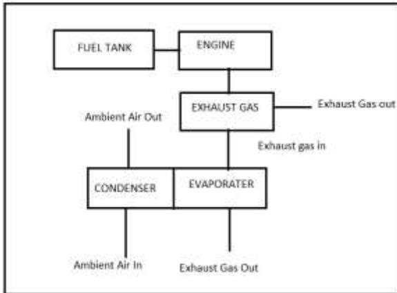
FIGURE 2 LINE DIAGRAM OF EXPERIMENTAL SET-UP
