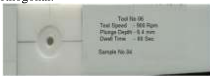
(a) single Spot welding specimen
