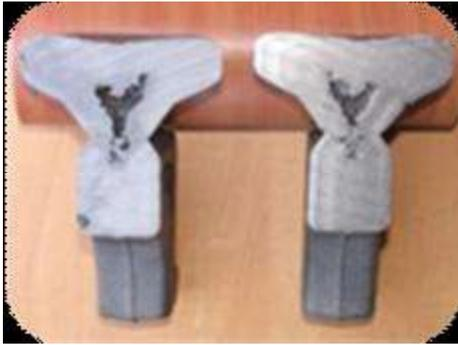
Fig.1 Shrinkage defect
