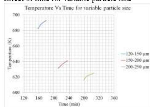
Fig 7: Effect of time for variable particle size
