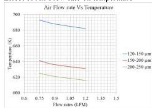
Fig 5: Effect of Air Flow Rate on temperature
