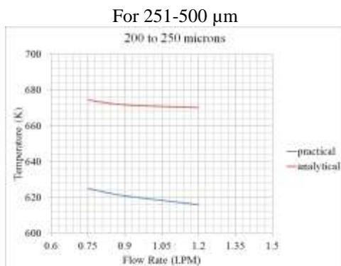
Fig 11: Analytical and practical comparison for 201-250 $\mu\text{m}$
