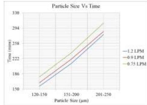
Fig 4: Effect of Particle size on time
