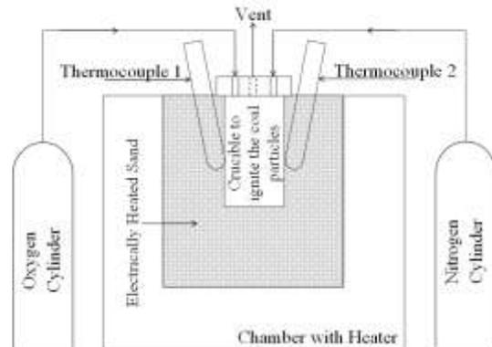
Fig 1: Schematic of coal combustion Setup
