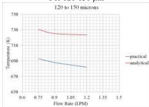
Fig 9: Analytical and practical comparison for 120-150 $\mu\text{m}$  For 151-200  $\mu\text{m}$
