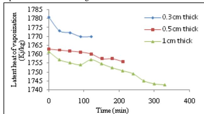
Fig 3: Typical variation of latent heat of vaporization with time for samples of different thicknesses and at drying air temperature of 60 °C
