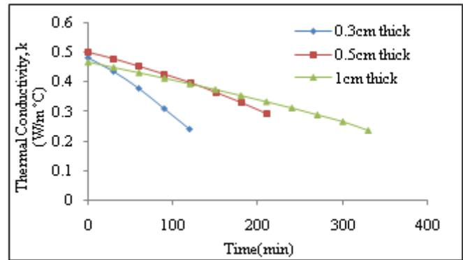
Fig 5: Typical variation of thermal conductivity, k with time for potato samples of different thicknesses and at drying air temperature of 60 °C.
