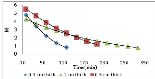
Fig 1: Moisture Evaporated vs. time for potato slices samples.
