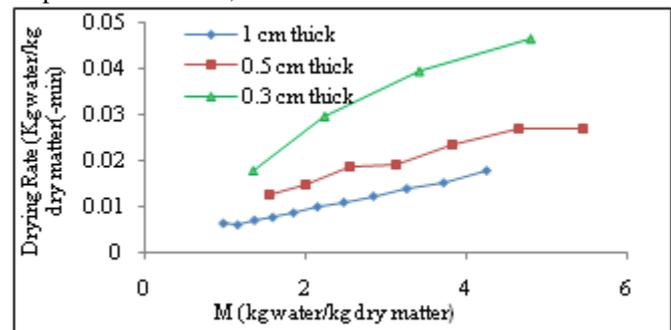
Fig 6: Drying rate vs. MC for potato slices samples of different thicknesses at drying air temperature of 60 °C.
