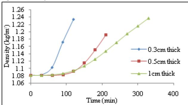
Fig 4: Typical variation of density with time for samples of different thicknesses and at drying air temperature of 60 °C.
