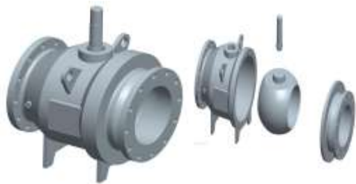
3D TWO PIECE SOLID MODEL OF BALL VALVE (As Per Existing Dimension DN300 (12")) Exploded View of ball Valve
