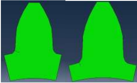
Backup ratio = 0.37, \theta = 80^\circ (Case 3) Backup ratio = 0.36, \theta = 80^\circ (Case 4) Crack propagation of 1mm in various spur gear models
