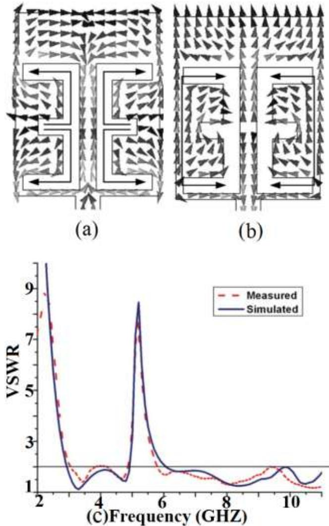
Fig. 4 Distributions of induced current in the Symmetric E-shape slot UWB antenna at the frequencies of (a) 5.2 GHz and (b) 7 GHz and (c) VSWR plots of the proposed planar monopole antenna [6]
