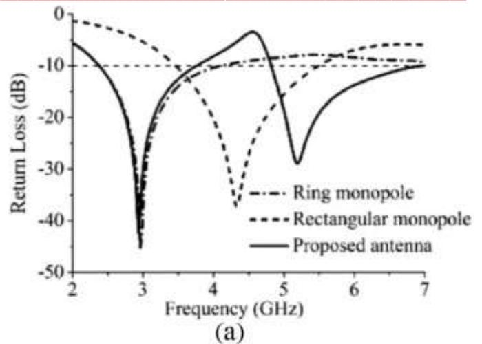
Fig. 2 (a) Return loss plot of the proposed Rectangular combined ring antenna [4]
