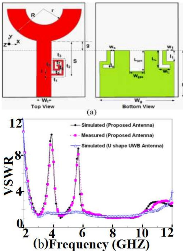
Fig. 5 (a) Compact printed dual band-notched U-Shape UWB antenna and (b) its VSWR curve [7]
