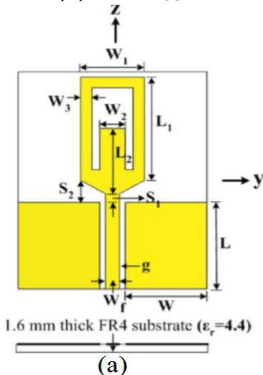
Fig. 1 (a) Geometry of Rectangular combined ring dual-wideband antenna [4]
