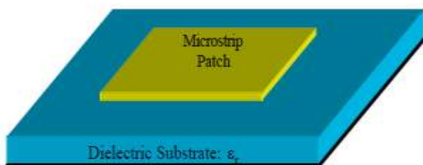
Fig. 1.1 Simple Structure of Micro strip Antenna
