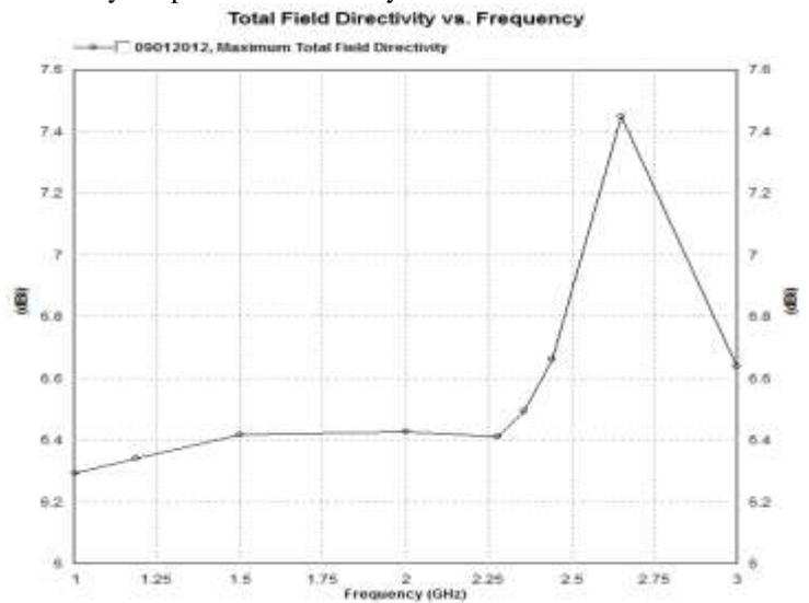
Figure.5.1 Directivity of Single Element Patch Antenna
