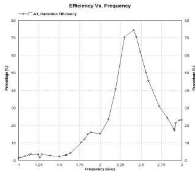
Figure.5.7 Radiation Efficiency of Patch Antenna Array
