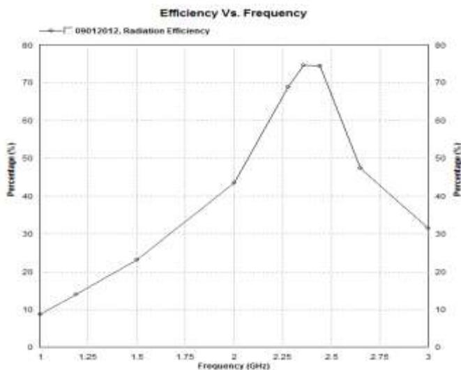
Figure.5.8 Radiation Efficiency of Single Element Patch Antenna
