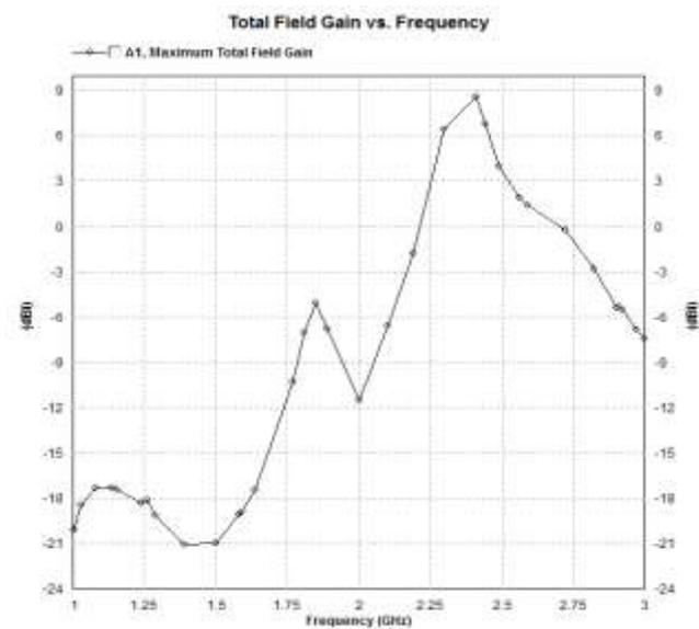
Figure.5.3 Gain of Patch Antenna Array
