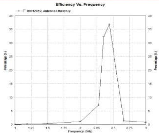
Figure.5.5 Antenna Efficiency of Single Element Patch Antenna
