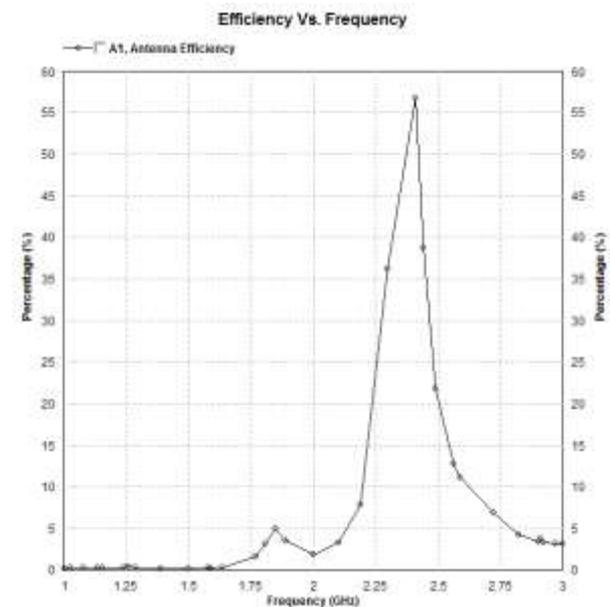
Figure.5.6 Antenna Efficiency of Patch Antenna Array
