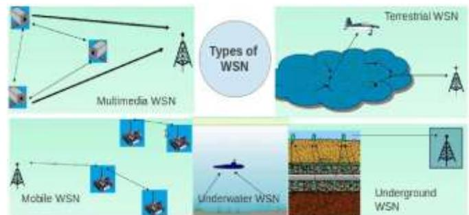
Fig. 2:Types of Wireless Sensor Network(WSN)
