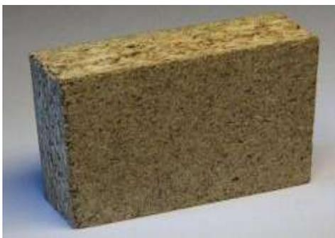
Fig. Bagasse Particle Board
