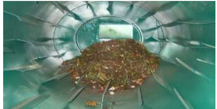
Figure 4: Internal view of rotary composter with baffle
