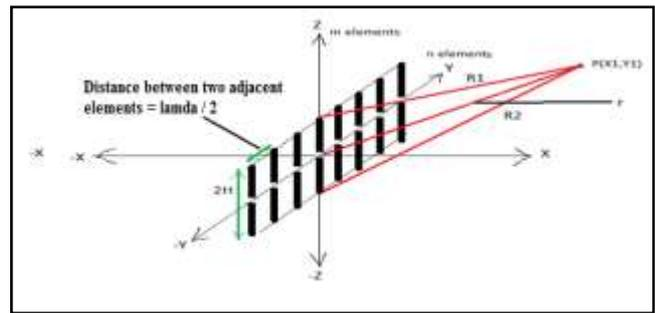
Figure 2: Field calculation of dipole array antenna at a point on the model
