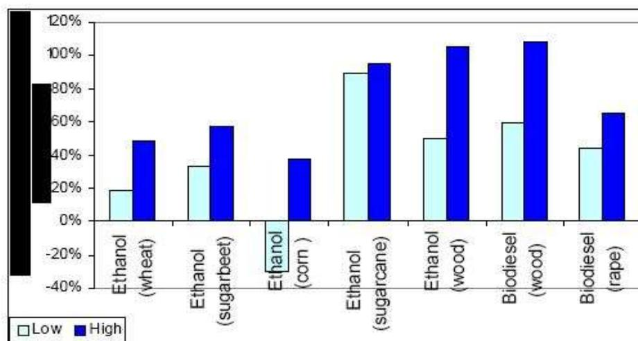
Figure 3 GHG reductions for different biofuels
