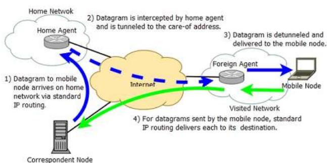
Figure 1: Operation of Mobile IPv4 Datagram Route.
