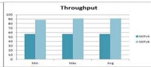
Figure 11: Throughput with tuned TCP window size 64kbytes during 3 minutes.
