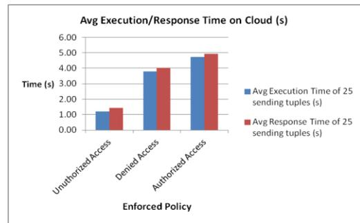
Figure 9. Execution time results of many trial access requests on cloud
