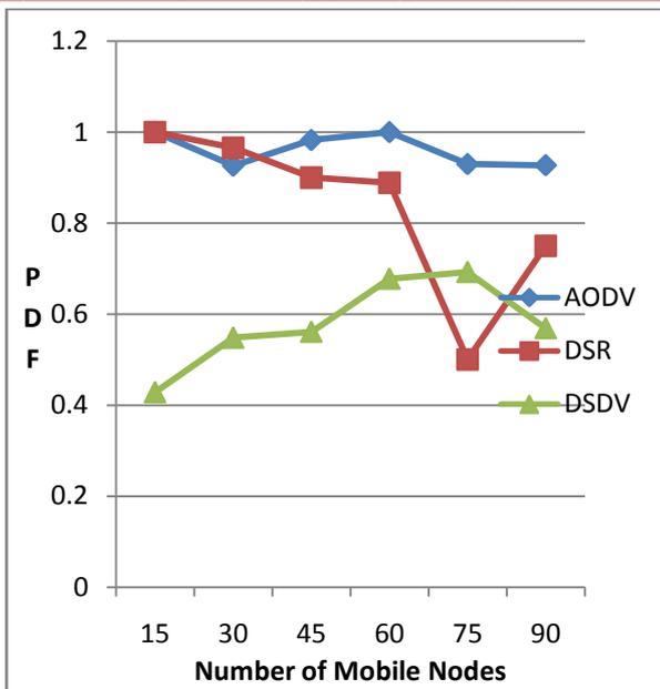
Figure 4: PDF versus No. of Mobile Nodes for AODV, DSR and DSDV
