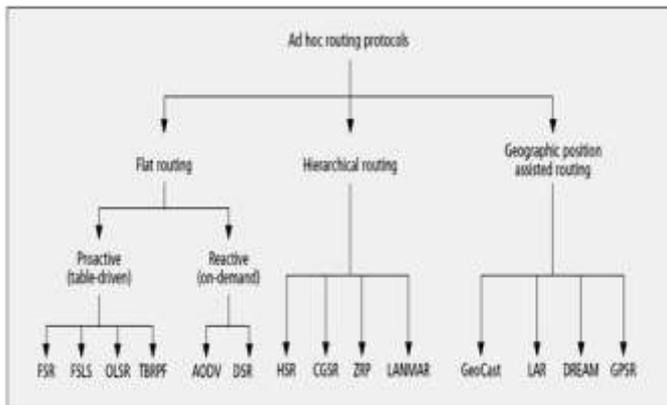
Figure 3.1: Classification of Routing Protocols in Mobile Ad-hoc Networks [2]
