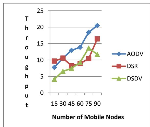
Figure 3: Network Throughput vs No. of Mobile Nodes for AODV, DSR and DSDV
