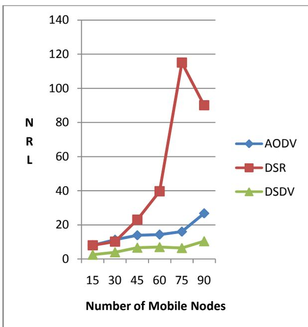
Figure 5: Normalized Routing Load vs No. of Mobile Nodes for AODV, DSR and DSDV
