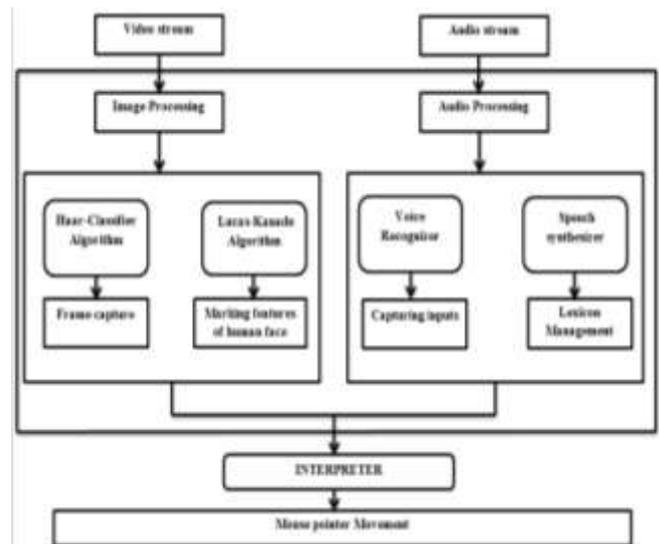
**Fig. 4.1: Proposed System Architecture**
