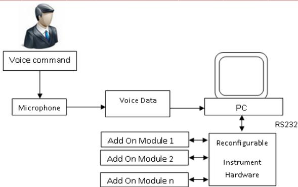
Figure 1. Block diagram of RVI
