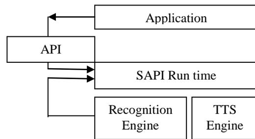
Figure 3. Block diagram of Speech application programming interface (SAPI)
