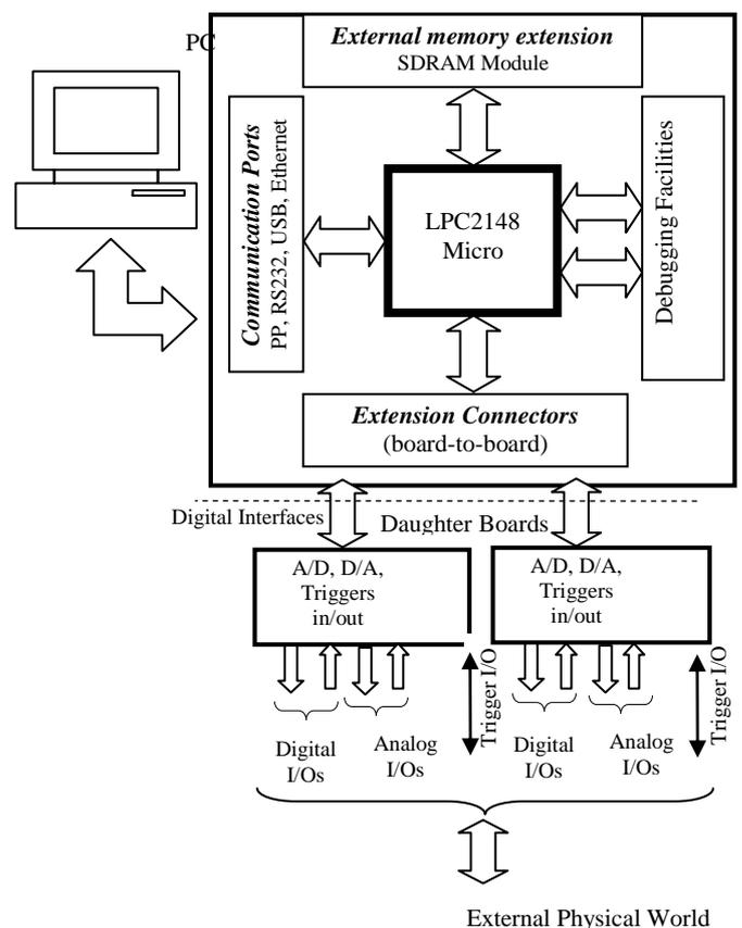
Figure 4. Block diagram Hardware Kernel RVI Main Board
