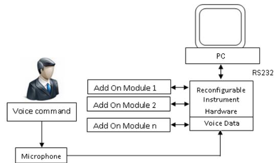
Figure 2. Block diagram of Speech controlled RVI
