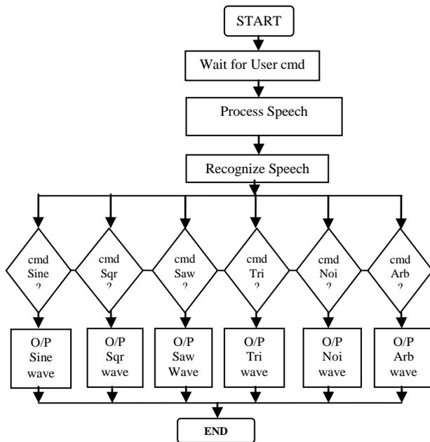
Figure 6. Figure6. Algorithm for function generator VI control
