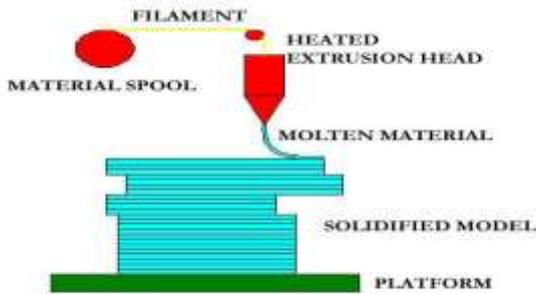
Fig 3: Molten material coming out of nozzle and deposited layer by layer.
