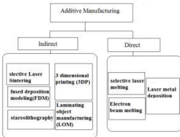
Fig 1: Different Additive Manufacturing Technologies
