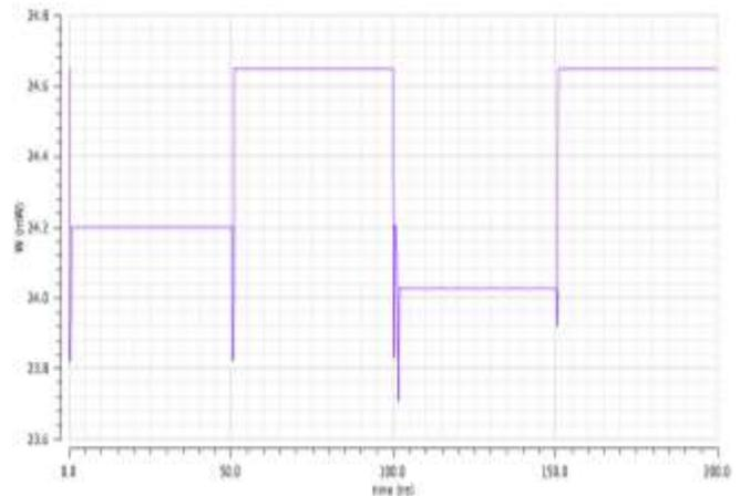
Figure 4. Proposed 8T SRAM Power Response
