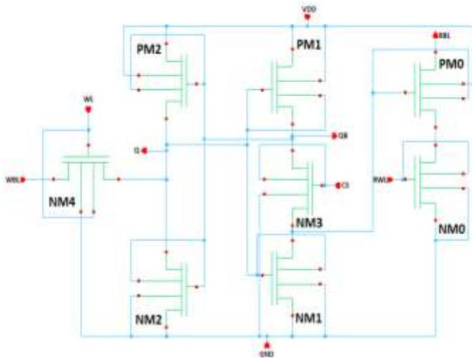
Figure 2. Proposed 8T SRAM Schematic
