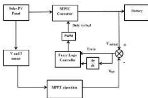
Figure 2. SEPIC converter with FLC controller and MPPT algorithm
