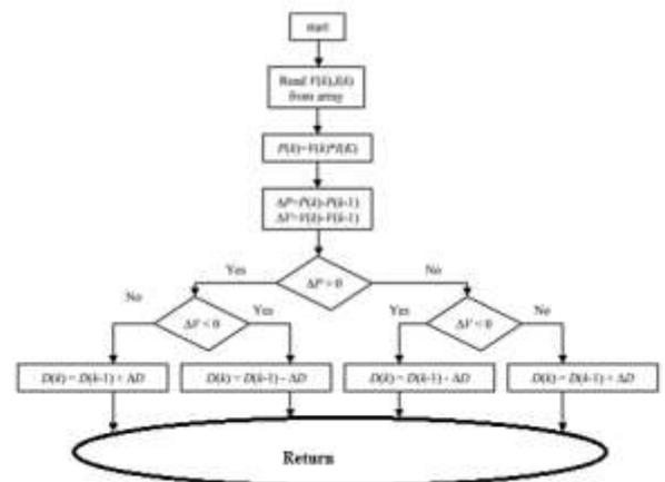
Figure 4. The flowchart of the Perturb and Observe Algorithm.
