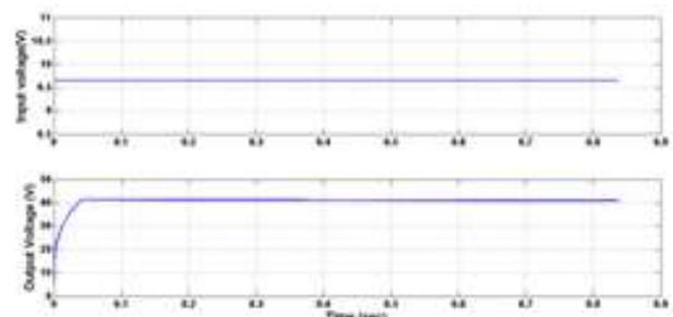
Figure 9. Input and output voltage of SEPIC converter
