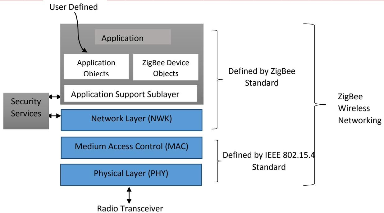
Fig 1: Relation between ZigBee and IEEE 802.15.4
