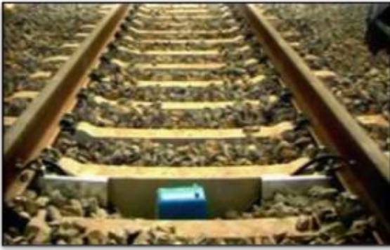
Figure-10. Transducer for Signaling System
