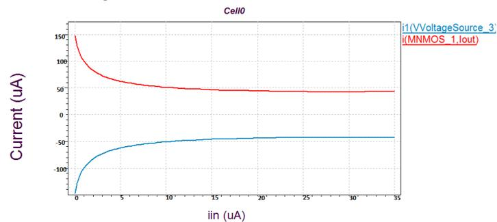
Fig 14: Simulation Results of Wilson Current Mirror
