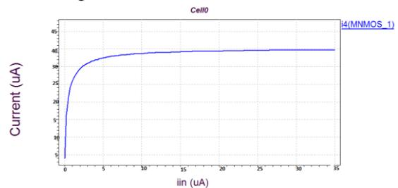
Fig 8: Simulated result for Cascode current mirror
