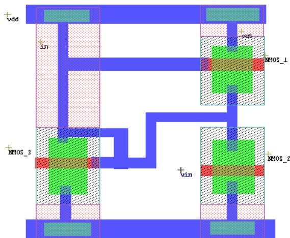
Fig-6 Layout of Conventional Regulated Cascode current mirror circuit designed in L-edit using N-channel MOSFET
