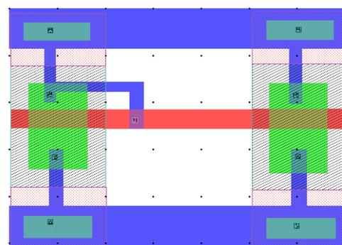
Fig 3: Layout of for simple current mirror designed in L-edit using N-channel MOSFET
