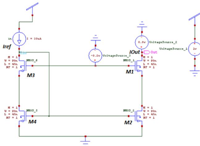
Fig 16: low voltage current mirror circuit
