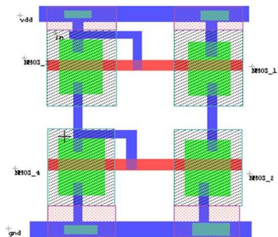
Fig- 9 Layout of Cascode current mirror designed in L-edit using N-channel MOSFET
