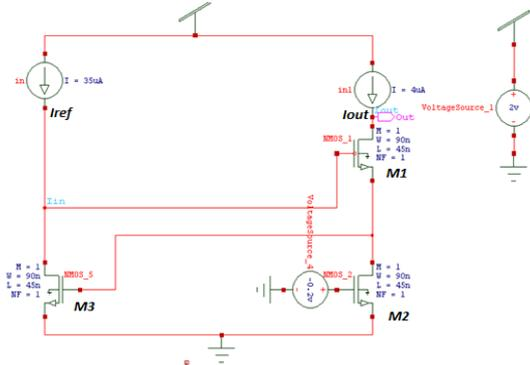
Fig 4: Conventional Regulated Cascode current mirror circuit
