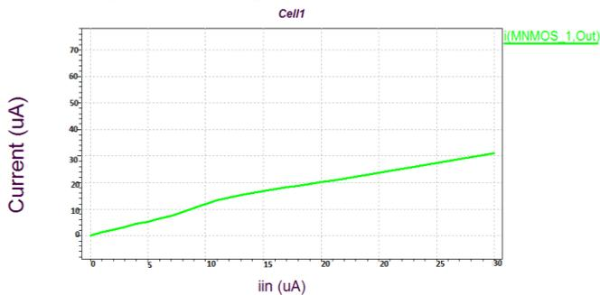
Fig 17: Simulation Results of low voltage Current Mirror
