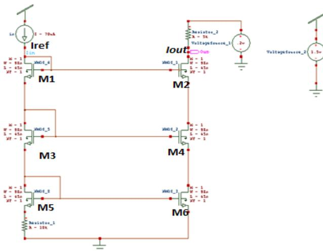
Fig 10: Triple Cascode current mirror circuit
