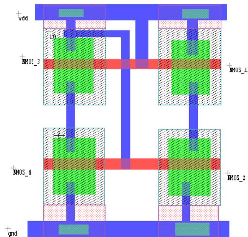
Fig-18 Layout of low voltage Current Mirror designed in L-edit using N-channel MOSFET
