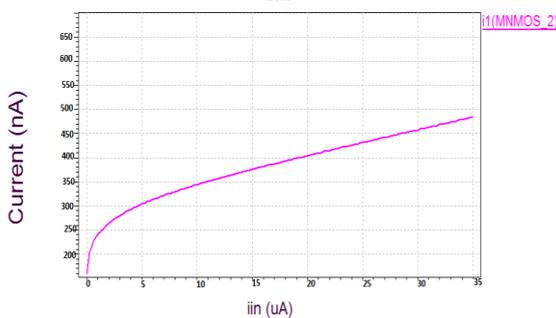
Fig 5: Simulated result for Conventional Regulated Cascode current mirror circuit
