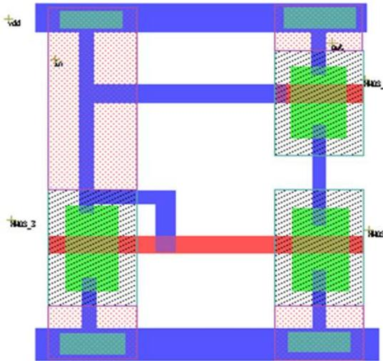
Fig-15 Layout of Wilson Current Mirror designed in L-edit using N-channel MOSFET
