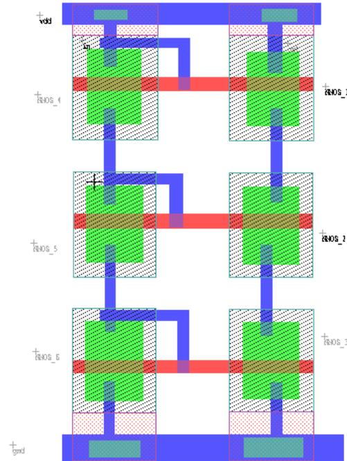
Fig – 12 Layout for Triple Cascode current mirror designed in L-edit using N-channel MOSFET
