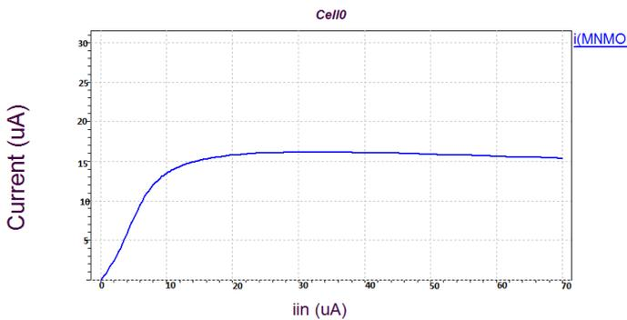
Fig 11: Simulated result for Triple Cascode current mirror
