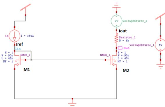
Fig 1: Simple current mirror circuit
