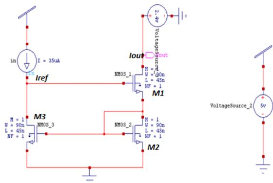
Fig 13: Wilson current mirror circuit
