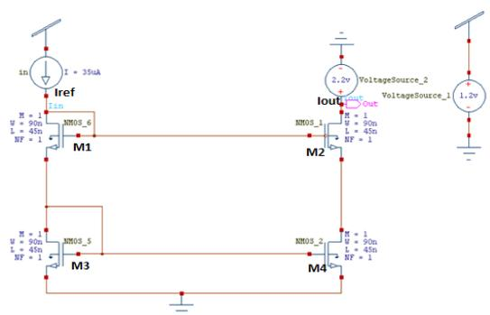
Fig 7: Cascode current mirror circuit
