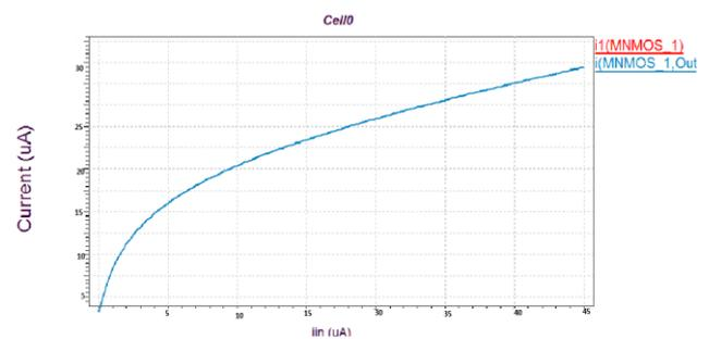
Fig 2: Simulated wave for simple current mirror
