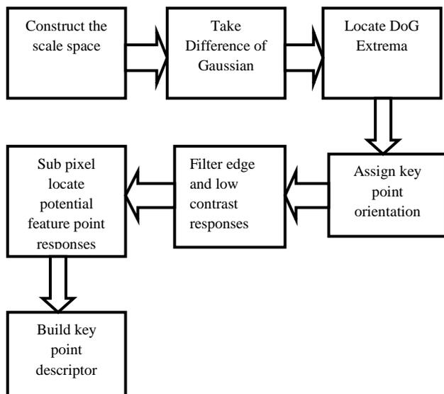
Fig. 2. Design flow for SIFT Algorithm
