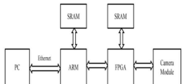
Fig.1 Block diagram of Image Acquisition System
