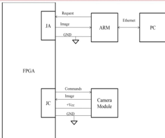
Fig.3 Communication between system devices
