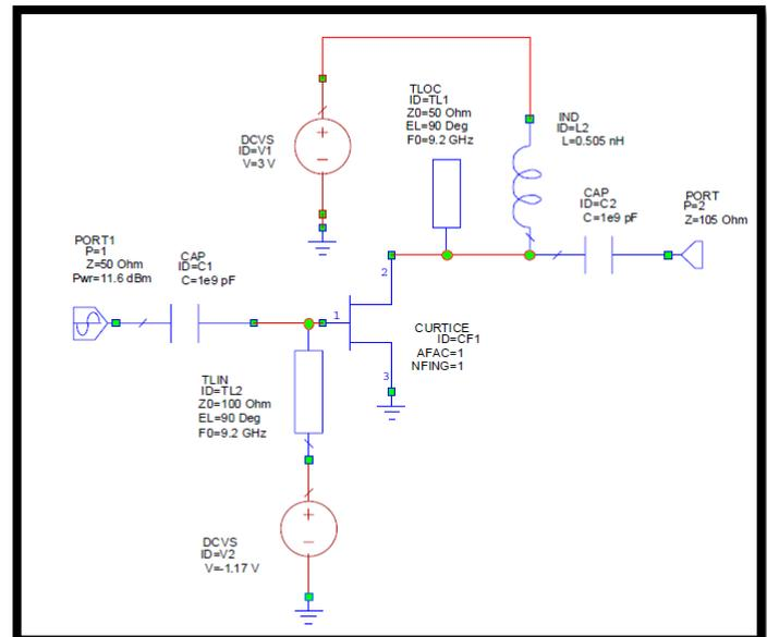
Figure 2.2: ideal circuit of active frequency multiplier [3]
