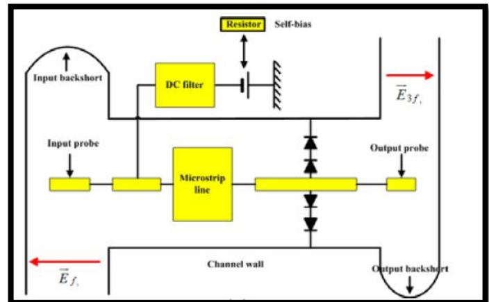
Figure 3.3: block diagram of unbalanced tripler with bias circuit [11]
