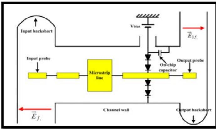
Figure 3.1: block diagram of common balanced tripler [11]
