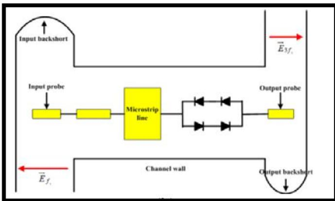
Figure 3.2: block diagram of tripler without bias circuit [11]
