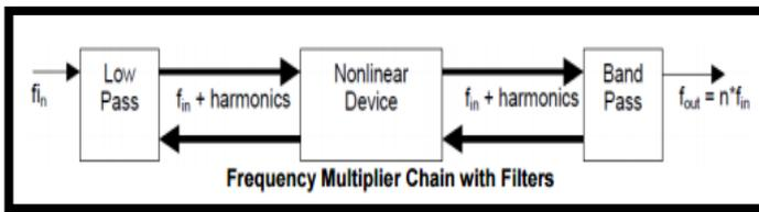
Figure 2.1: frequency multiplier basic block diagram [2]
