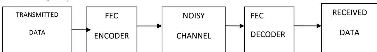
Figure1.1 forward error correction concept
