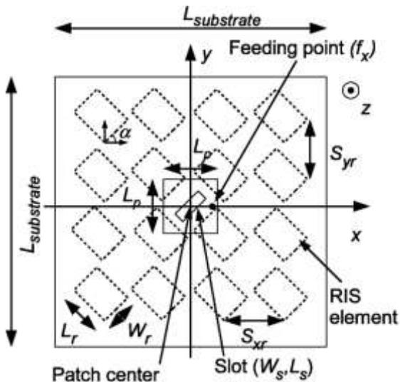
Figure 9. Top view of proposed slot antenna on RIS [20]
