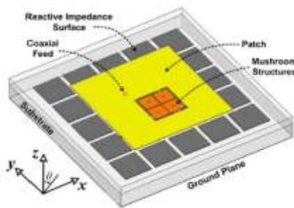
Figure 5. Perspective view of a proposed CP patch antenna with RIS & mushroom like CRLH[16]
