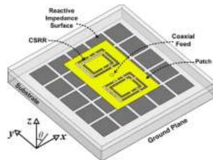
Figure 6. Perspective view of a proposed CP patch antenna with RIS and CSRR[17]
