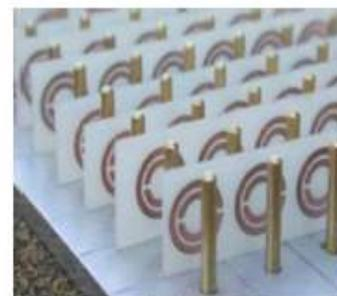
Figure 1. Combination of Alternating Layers of Thin Metallic Wires and Circular Split Rings
