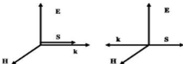
Figure 2. Left: Right Handed System and Right: Left Handed System [8]
