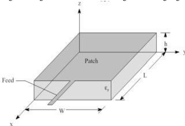
Figure 9: Geometry structure of rectangular patch [2]
