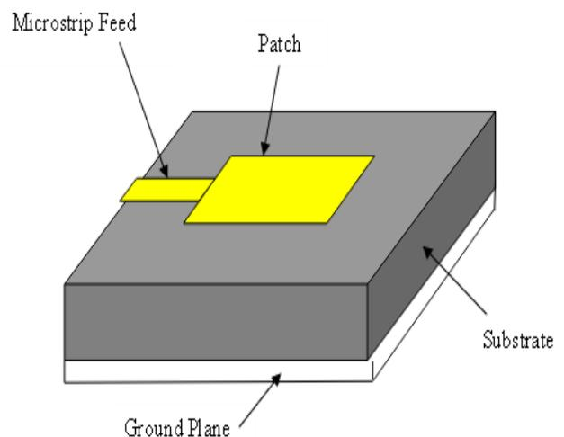
Figure. 4: Basic structure of Microstrip patch antenna [2]
