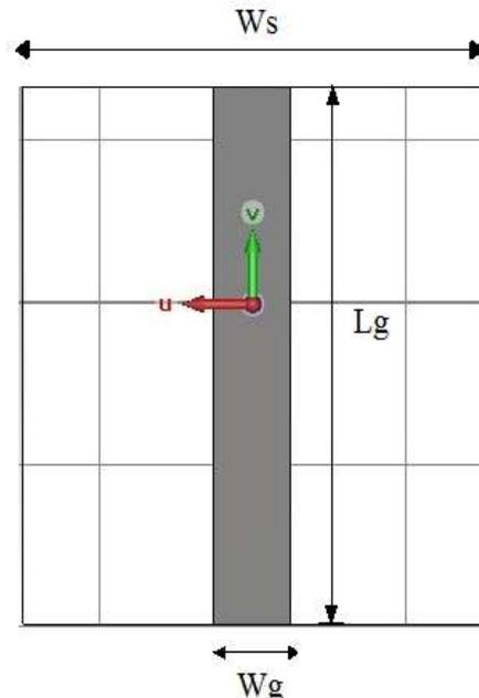
Figure 7: Defected ground structure
