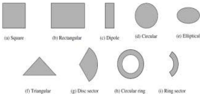
Figure 5: Different shapes of patch mostly used in microstrip patch antenna [2]
