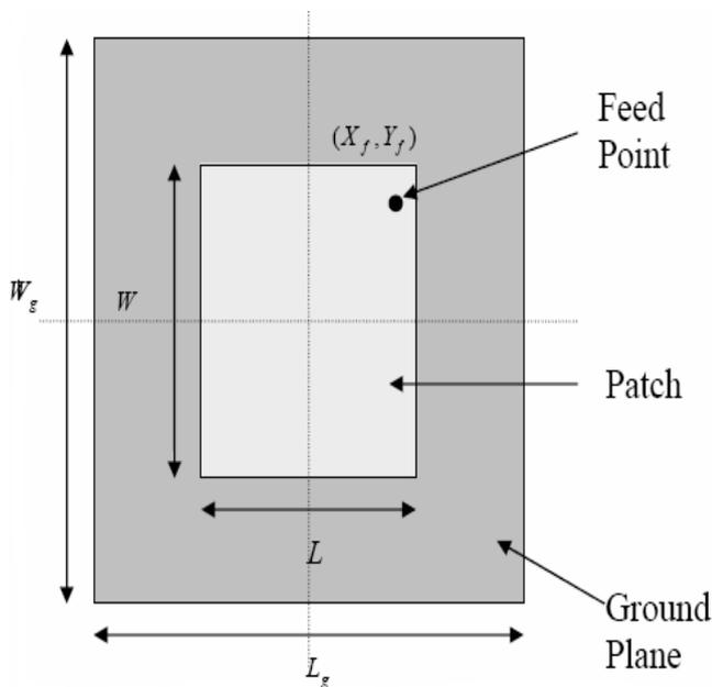
Figure 6: Basic structure of rectangular patch
