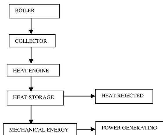
Fig.1 Schematic diagram of a solar thermal conversion system
