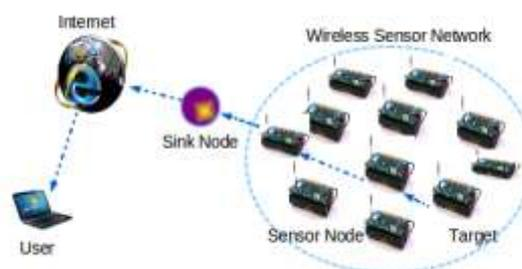
**Figure 1.1 Basic structure of Wireless Sensor Network**
