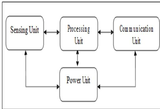
**Figure 1.2 Basic Building Blocks of Sensor Node**
