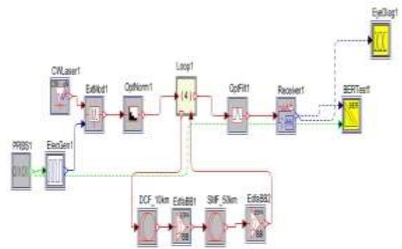
Figure 2 Simulation setup of an optical communication system consisting of DCF for nonlinearity mitigation
