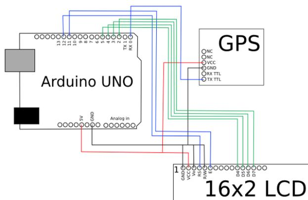
Fig.2 GPS and LCD are connected with ARDUINO
