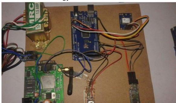
Fig.4 Hardware of Bike Dashboard Unit
