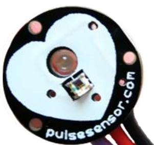
**Fig. 2- Above figure represents pulse sensor**
