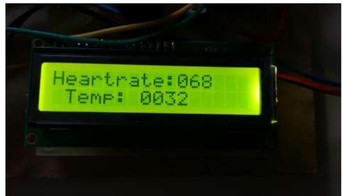
Figure 2. Heart rate & Body Temperature displayed on LCD Display
