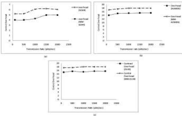
Figure 2. Overhead comparison of (a) SOAR, (b) AOMDV and (c) OLSR routing protocol for variable transmission rate.
