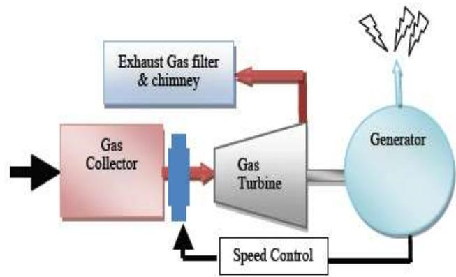
Figure 3. Schematic diagram of generation unit
