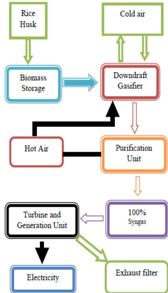
**Figure 1. Block diagram of a rice husk electricity production unit**
