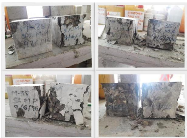
Fig 2: Cubes after Compression test
