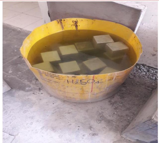
Fig 5: Cubes dipped in Sulphuric acid
