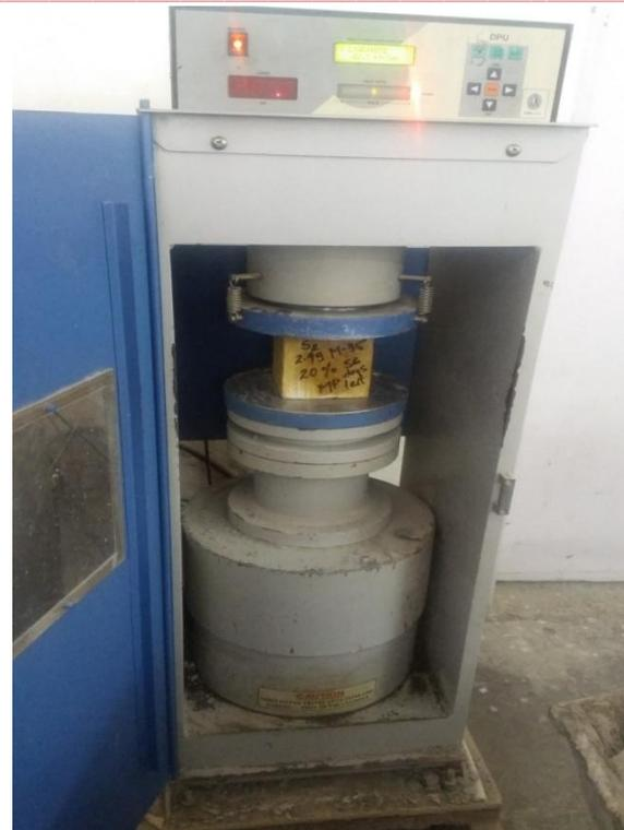
Fig 3: Compression Testing Machine
