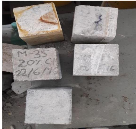
Fig d: cubes dipped in different solution after 28 days
