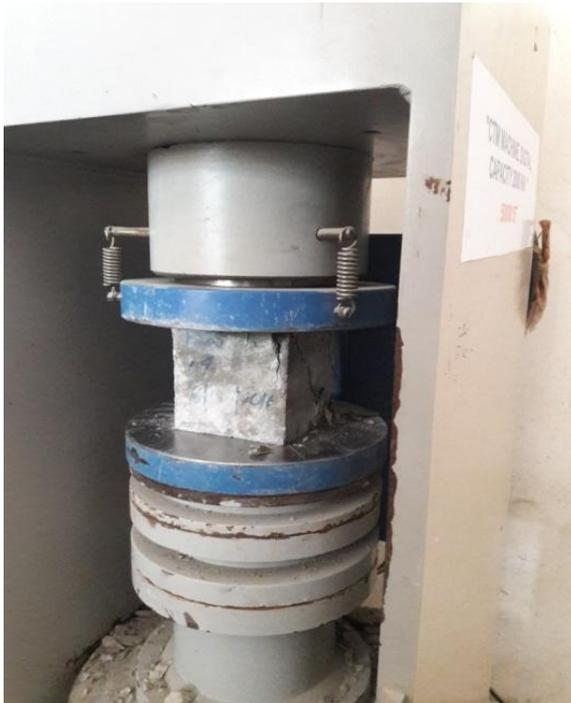
Fig c: Compression Testing machine
