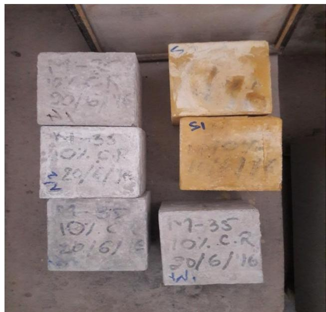
Fig e: cubes dipped in different solutions after 56 days
