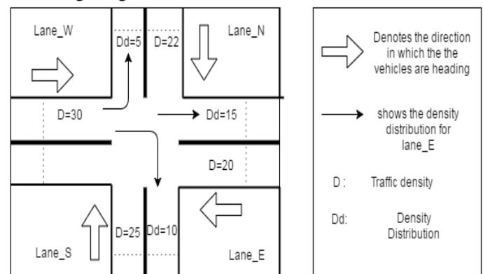
Figure 3. Traffic Distribution and traffic density capture
