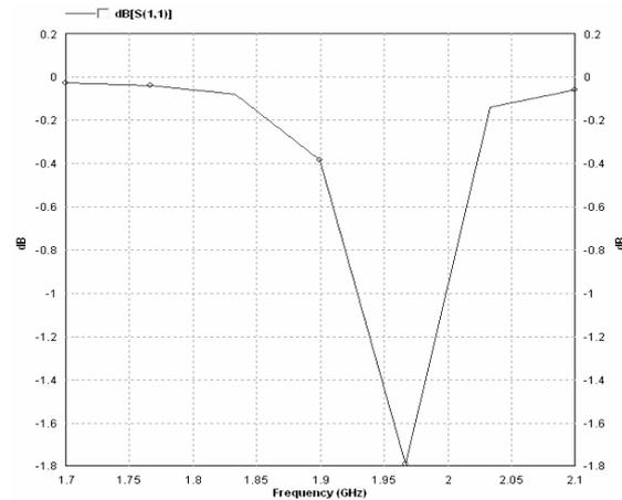
**Fig.3.8.return loss curve for substrate height =0.5mm**
