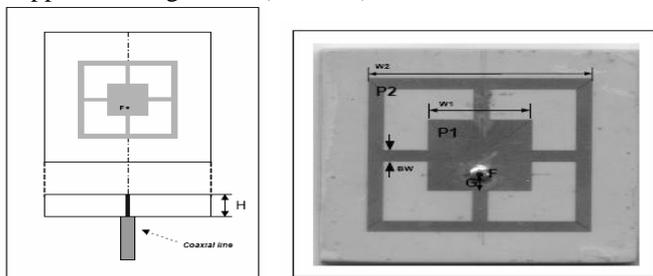
**Fig.3.10 Configuration of the dual band patch**
