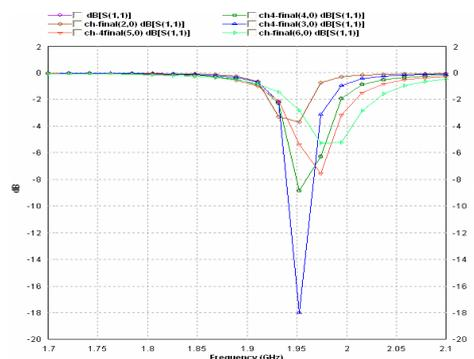
Fig.3.4. Return Loss curve for different feed points
