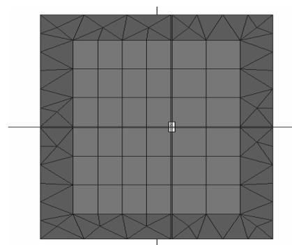
Fig.3.3 The meshed patch designed in IE3D to resonate at 1.9 GHz In this case the probe is located at (2,0)
