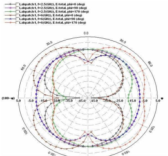
**Fig.3.9. Polar plot for the antenna for three values of  $\phi$  at  $f=2.5\text{GHz}$  and  $f=6\text{GHz}$**
