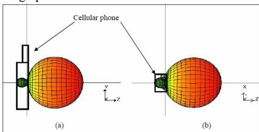
Fig 3.2 (a) 3D view of radiation pattern for cellular phone orientation in the YZ plane (b) 3D view of radiation pattern for cellular phone orientation in the XZ plane
